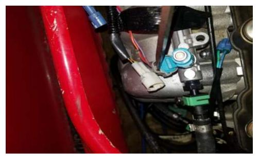
14. Remove connectors on fuel injectors. These can be very difficult to remove. You can very carefully use the flat head screw driver to pop up the clip tab to pull off easier.
