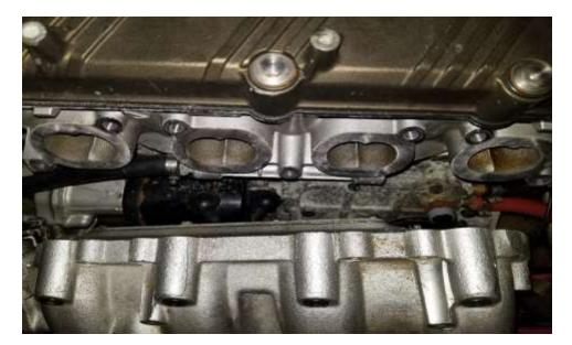
29. Remove reminder of studs. Make sure the face of the exhaust ports are clean of all gasket material and oil. You may need to block off all ports with paper towels and use the razor blade to scrape. Scotch brite may be needed also, this must be bare aluminum to seal properly. Blow with air and wipe with brake cleaner to remove oil when done.
