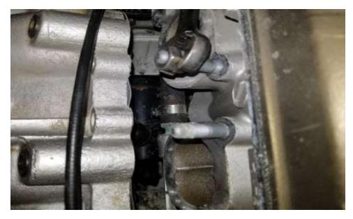
27. Using the bottom nut only and the 13mm open end wrench, loosen the stud.
