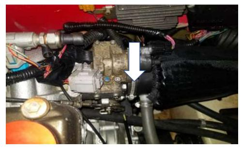
2. Locate the hose clamp holding the air filter or hose on to the throttle body.
