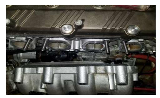
31. Place the four studs in the 4 top threads as show. Screw in by hand only.
