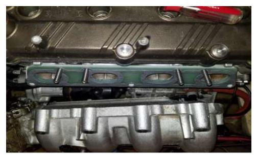
34. Place the second gasket on top of the barrier, again gasket side does not matter.
