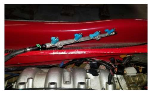
16. Remove the fuel rail out of the way.
