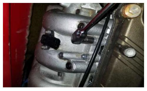
20. Remove the acorn nuts on the intake manifold using an 12mm socket.
