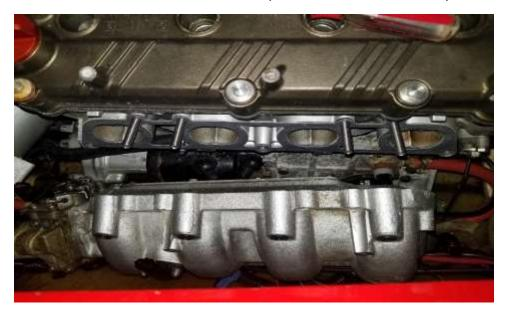
32. Place the gasket on the engine, side does not matter.
