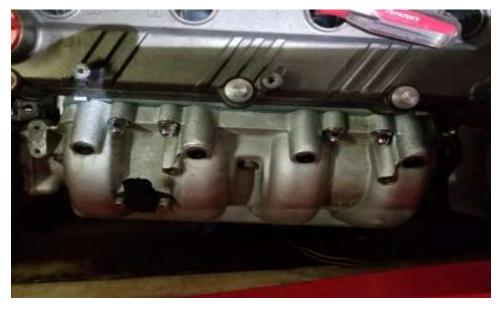
36. Place your washers and acorn nuts on the four studs, and 3 short bolts with washers as well. Tighten acorn nuts to 14 ft.lb and bolts to 18 ft.lb.
