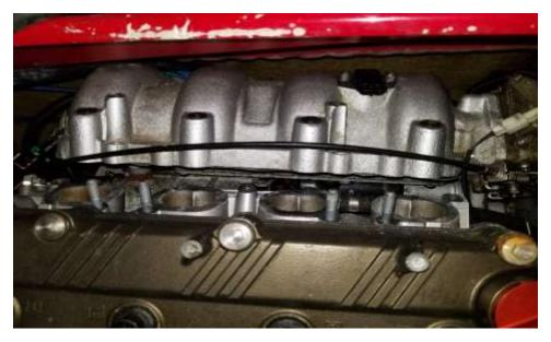
24. Remove manifold and set down in hull. A rubber mallet may be required to tap the manifold free.
