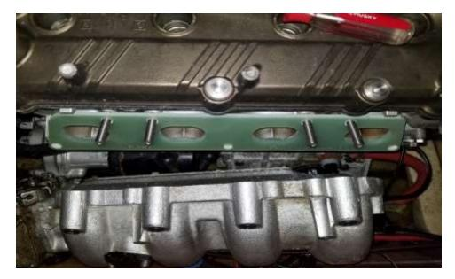
33. After the gasket has been place on, place the thermal barrier on. Make sure the Kawi Performance logo faces you as shown.
