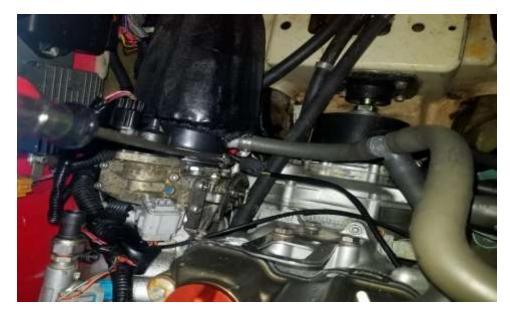
3. Remove filter with long flat head screw driver.
