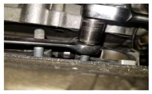
26. Using a 13mm wrench and a 13mm socket, tighten the two nuts together as much as possible.
