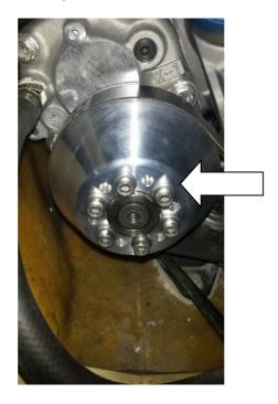
2) Using OE Spring Retaining Bracket, compress the spring enough to slide the bracket on. Remove tension, this will remove tension off your belt. NOTE: Not using this bracket can permanently damage your tensioner!
