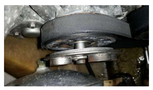
8) After all screws are removed, you can now remove the damper. This should slide forward easily. If not, a screwdriver and penetrating oil may be necessary.
