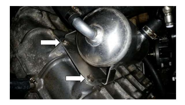
3) Remove the two M10 bolts holding the oil separator in place.
