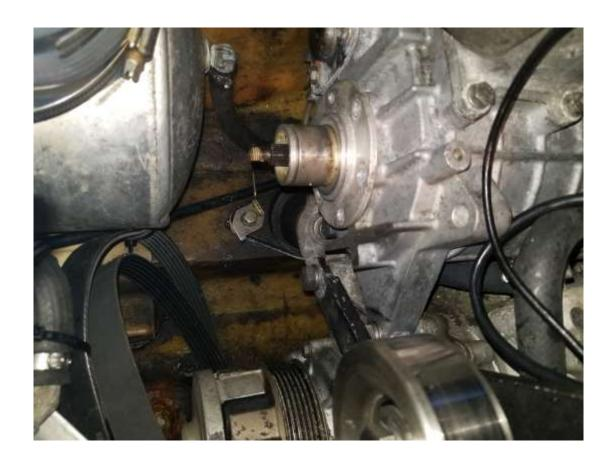
12) Remove hub with a screw driver, it should pry off very lightly if this is a R&D hub. If this is OEM or KP you must heat it with a torch and pull it off with plyers. Remove all corrosion/ silicone if present.
