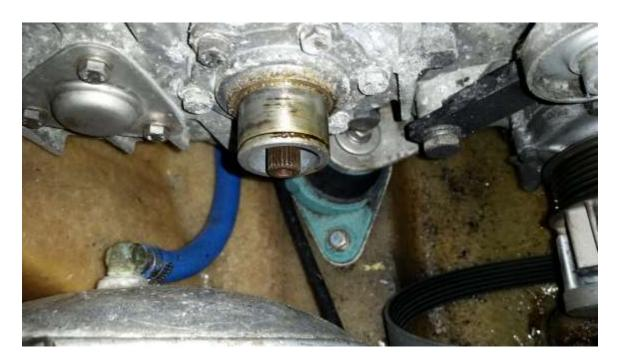
11) Remove screws on hub as shown below.
