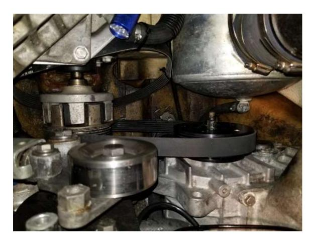
20) Install Damper. Apply red Loctite to all cap screws.
