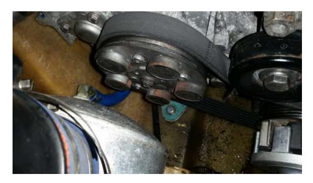
5) Depending on the condition of your pulley/supercharger, you may need to remove the exhaust manifold and water box. Please refer to Kawasaki service manual if this is required.
