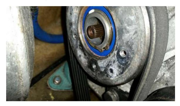
9) Remove damper. Next you will need to remove the snap ring. More than likely the snap ring will not be in your favor, and will be facing the other side. You will need to spin the snap ring. And use the tool to remove. At this point you can now remove the belt and tensioner. Please refer to service manual for tensioner removal.
