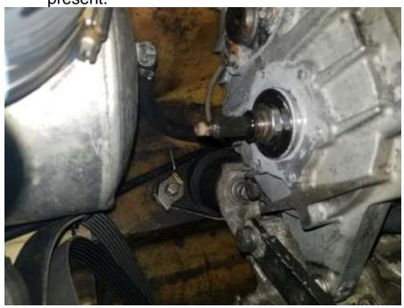
13) Using a torch heat the KP hub until it slides over the bearing. DO NOT heat more than 20 seconds! Note: You can apply a small bead of grey RTV silicone to the rear of the hub only to keep water out.
