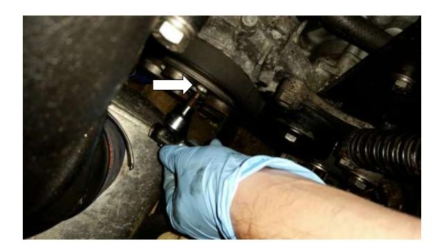
7) Remove all five socket cap screws. This is easiest with the tensioner still in place. NOTE: If your pulley is in rough shape make sure to remove water box and muffler first. This will save you a trip to the dealership, if you strip a bolt. You may need to hammer the tool into the socket cap screw to assure the screws do not strip.
