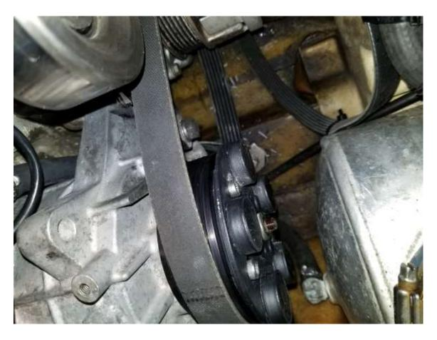
22) Install center bolt or acorn nut. Apply red Loctite. Torque bolt on older models to 11 ft.lb, 16 ft.lb on the acorn nut.
