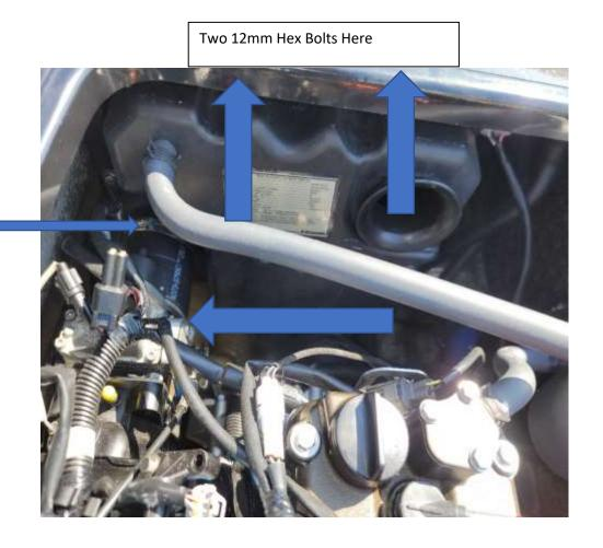
\*NOTE\* It may be difficult to remove air box from hull. You may need to remove the 10mm hex bolts and separate the box to remove from hull.
